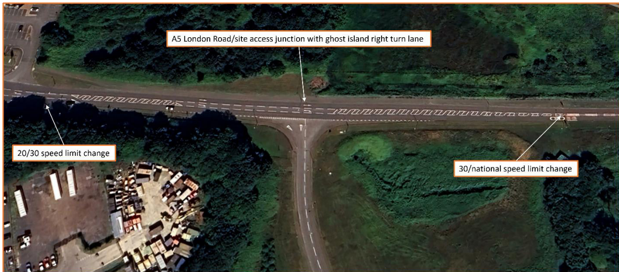
Figure 12: existing access junction
